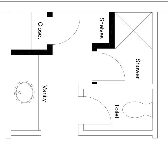
Second Floor Apartment Bath Floor Plan Scale: 1/2"=1'-0"
